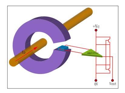
Principle: Hall devices are used to directly detect the primary magnetic field generated by the current in the primary conductor, Output voltage signal after linear amplification. Inside the sensor, special stability and temperature compensation circuit areadopted, Thus the outside voltage and temperature on the sensor to minimize the impact.
